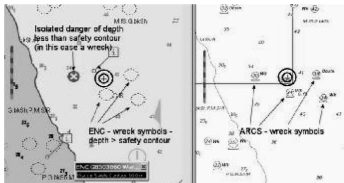
Fig. 1. An example of the use of the Isolated Danger symbol on an ENC
