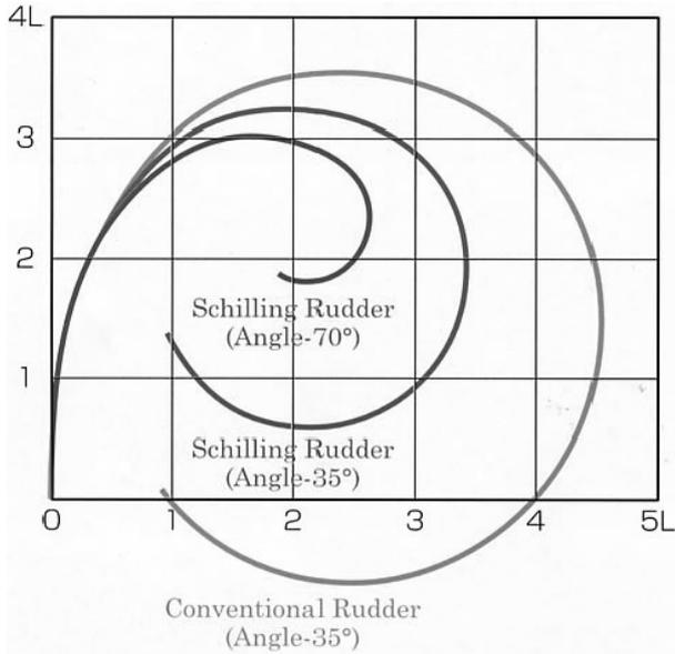
Fig. 2. Comparison of Turning test Results at Sea Trial (Japan Steering Systems)
