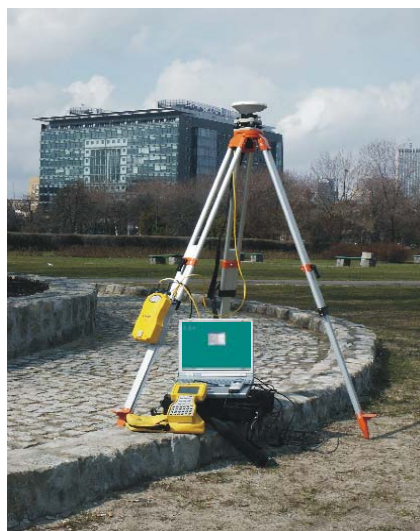
Fig. 1. Field set for RTK and DGPS measurements
