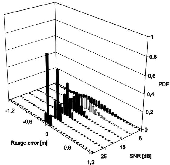
Fig. 5. PDF of range measurement error of the DVB-T signal
