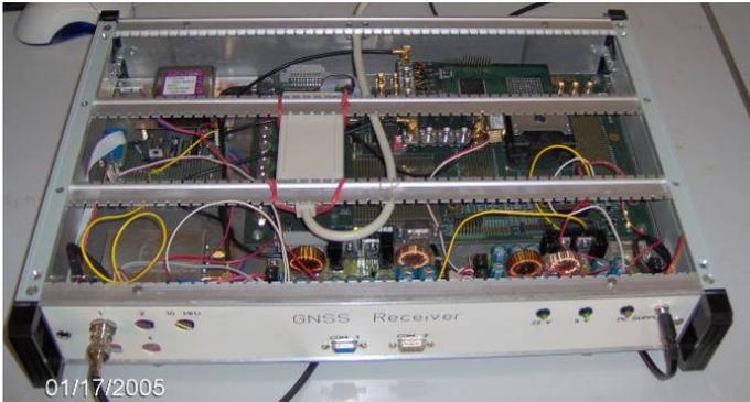
Fig. 3. Experimental GNSS Receiver in 19-inch rack
