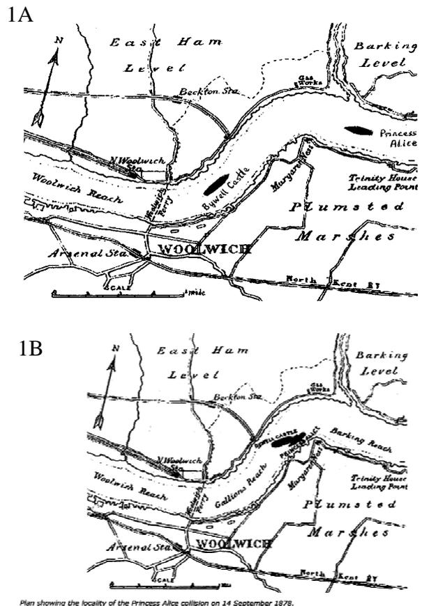
Fig. 1. The positions of the *Princess Alice* and the *Bywell Castle* at 5 minutes before the collision (1A), and at the time of the collision (1B), based on a contemporary chart
