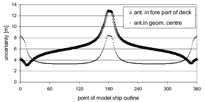
Fig. 6. Errors comparison of consecutive ship's outline points determined for INS using DGPS IALA position source and two synchronically working DGPS IALA receivers as a heading source with GNSS antenna situated in geometrical centre and out of it
