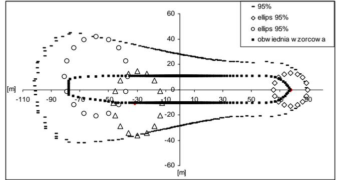
Fig. 3. The uncertainty area of ship's location around the model ship outline formed after extreme points of error ellipse had been found for 95% confidence level and antenna GNSS placed in fore part of the ship
