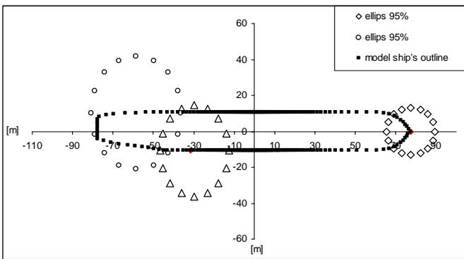
Fig. 2. The errors ellipses of chosen points the ship's shape outline is built from with semi-axes  $a = \sigma x_{ri}$  i  $b = \sigma y_{ri}$  formed in result of continuous line discretization into 16 points
