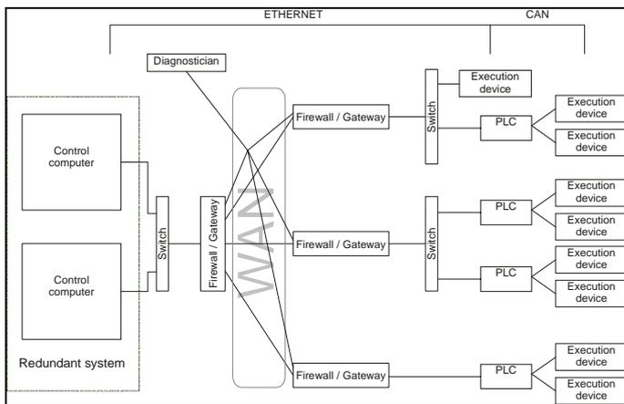
Fig. 1. Construction of a system with devices protecting against access of unauthorized persons
