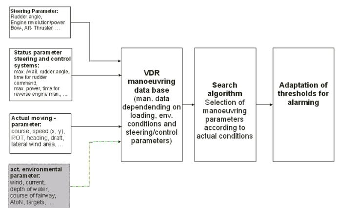
Fig. 7. Principal structure of the application of recorded manoeuvring data for self-adaptation of alarm thresholds
