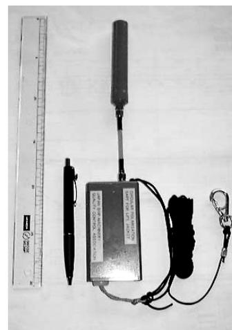
Fig. 4. SART for life jacket installation
