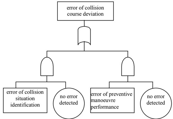
Fig. 5. Fault tree of collision course deviation
