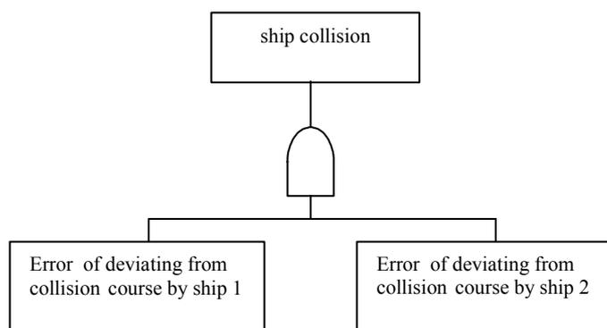
Fig. 4. Fault tree of ship collisions
